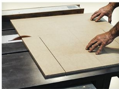
3 Instead of a circular saw, cut the notches in the MDF panels on a table saw.
