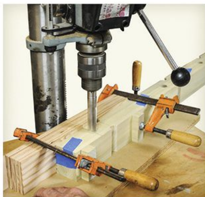
2 Clamp the uprights to the drill-press fence before boring the center holes.
