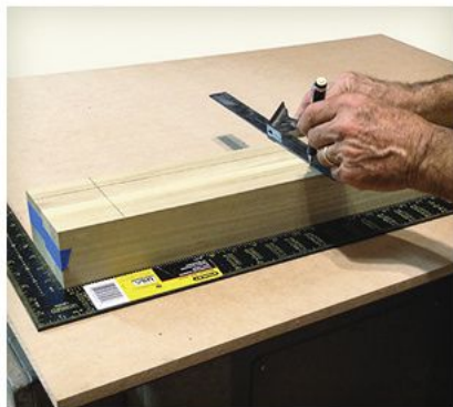
1 Tape the uprights together, use a square to align them, and mark each hole location.
